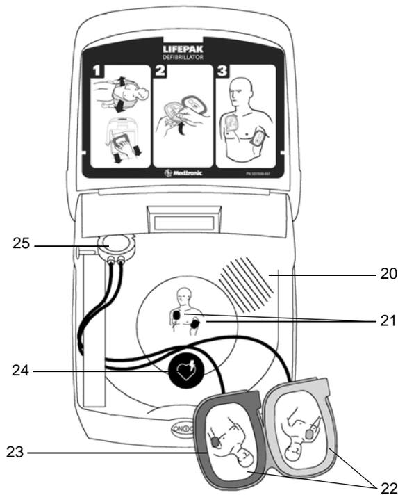
**Figure 4** Inside Features after Opening the Electrode Packet
